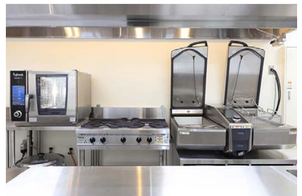
First-floor main kitchen. Equipped with a Vario Series Dual Pan, combi oven, gas range, etc.
