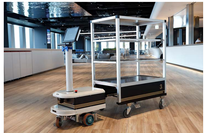
The autonomous transport trolley. A tablet-controlled robot (right photo) is pulling the trolley (left photo). The robot and trolley can be detached.
