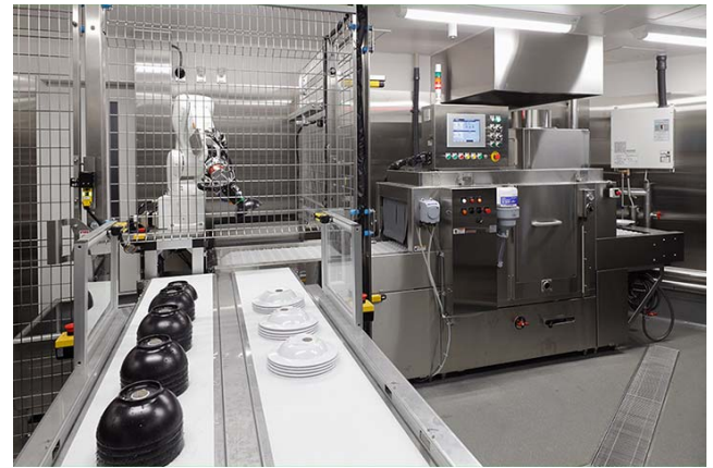
Photo shows “finibo,” an automatic dishware sorting robot. It recognizes washed dishes coming from the dishwasher on the right by the sensor, blows off the water from their bottom rims, picks them up, and sorts them in a specific order on the collection conveyor in the foreground.
