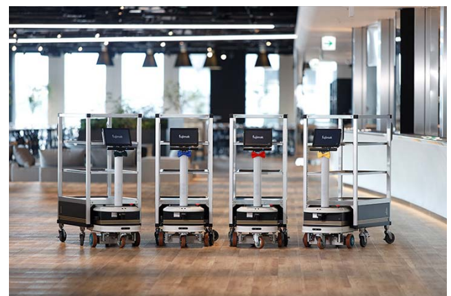
Four autonomous transport trolleys are in operation, each designed to resemble a concierge trolley. The outer plastic molding was designed by the Isuzu Motors Design Center.
